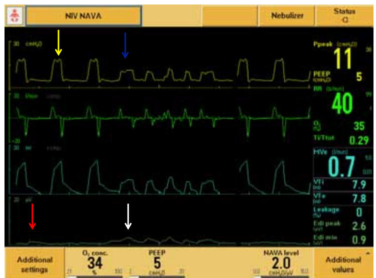
Figure 5: Edi set at 0.5 mcV. Small Edi signals are now ignored (red arrow) and the neonate remains in backup (yellow arrow) getting effective pressure control breaths. When a larger Edi signal is detected (white arrow), the neonate gets an adequate NAVA breath (blue arrow). Stein and Firestone, Neonatology Today 2012.
