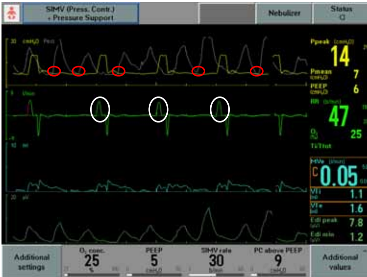
Figure 1: Failure-to-trigger -- This panel shows the pressure (first line), flow (second line) and Edi (fourth line) tracings in a neonate on SIMV (Press. Contr.). The Edi signal is converted to a pressure estimate (P.est) that is shown as a white line superimposed over the yellow pressure line in the upper tracing. The P.est represents what the pressure would be if the patient was in NAVA. In the upper tracing the patient appears to be apneic with no evidence of flow triggering (white circles) and is being ventilated in pressure control. The P.est represents the neonate's actual respiratory drive and demonstrates that there is a strong respiratory drive that is not detected by the flow trigger (red circles). Stein and Firestone, Neonatology Today 2012.
