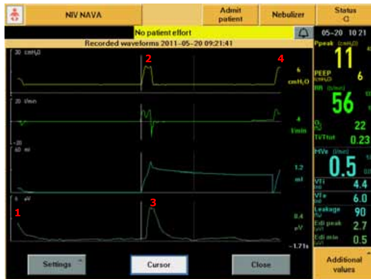
Figure 7: The neonate has a spontaneous breath (1) and then becomes apneic. After 5 seconds of apnea the neonate receives a backup breath (2) that generates an Edi signal (3). This is Head's Paradoxical Reflex and is secondary to diaphragmatic expansion and not a signal from the phrenic nerve. Although the Edi signal is not converted into a breath, the apnea timer has been reset and the neonate remains apneic without ventilation another 5 seconds before the next backup breath occurs (4) Stein and Firestone, Neonatology Today 2012.
