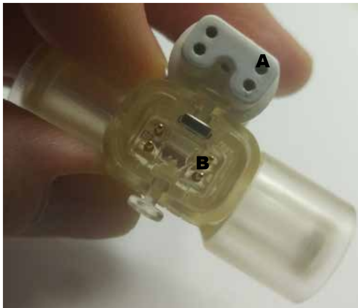
Figure 5: hot wire anemometer and connecting cable. A: Look for damage or discoloration (usually greenish) here as it may affect signal quality. Look for corrosion at the base of the connecting pins. B: The cable should connect such that it is at the top of the sensor.
