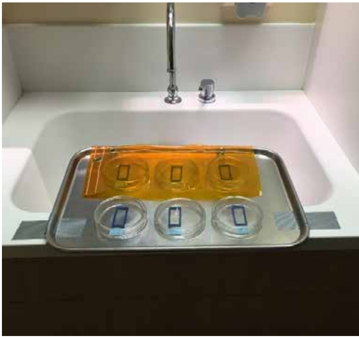
Figure 6. Inoculated culture plates at patient room sink (left) and counter (right); borosilicate glass covered all test plates, and additional orange-colored UV-blocking film covers each control group.
