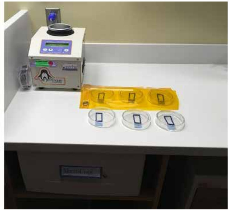
Figure 6. Inoculated culture plates at patient room sink (left) and counter (right); borosilicate glass covered all test plates, and additional orange-colored UV-blocking film covers each control group.
